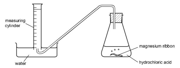
The flask contains 1cm length of magnesium ribbon and 25 cm<sup>3</sup> of hydrochloric acid.
